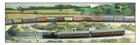
The whole layout is operated from one side, three operators is ideal. There are both electric points and wire powered ones. The main control board has a bewildering array of switches allowing each of the four tracks to be driven independently. Hammant and Morgan controllers were used but a couple of these units have failed and are replaced by Gaugemaster controllers.
